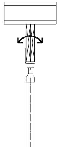
**Remember: Column top plates/saddles are to be bolted (1/4" x 3" lags) to the supported wood beams.**
